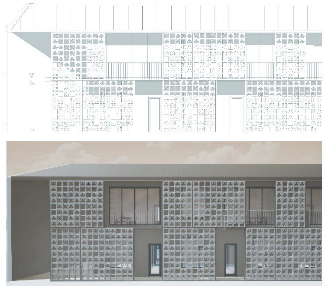
Fig. 6. Design study in Gyöngyös, perforated facade with grape leaf motifs. (Source: own design, cons.: Zsófia Mádiné Dankó DLA, 2023)
