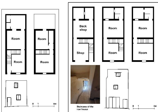
Fig. 19. Plans Elevations of row houses; in the two examples, the top-floor window is the only one centred. On the lower floors, the window is off-centre, as the vertical circulation has been subtracted from the width of the front cell. (Source: Authors, 2024)
