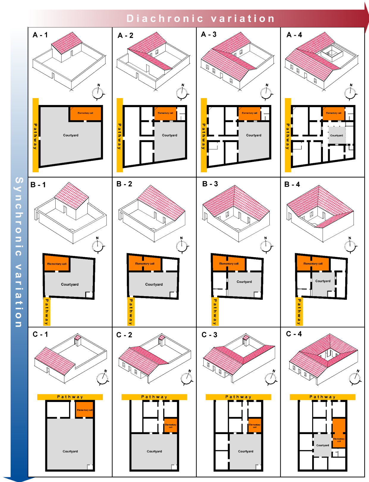
Fig. 13. Typological process of the courtyard house. The table summarises the variants of the single-family house within the limits of the original plot and with minimal specialisation: (A-1) entrance and path to an elementary cell perpendicular to the street. With the best orientation, this room remains, throughout the process, the main space of the house, i.e. the family living room; (B-1) elementary cell opposite the entrance and leaning against the back wall; (C-1) entrance from the covered part built alongside the street. Columns 2, 3 and 4 represent the successive phases of growth through progressive occupation of the open sides of the enclosure. (Source: Authors, 2024)
