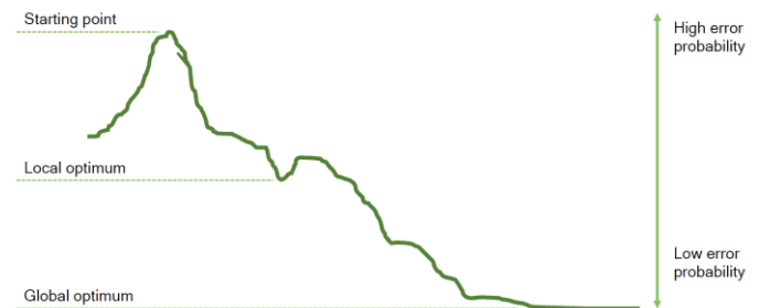
Figure 6: Overcoming problems with ANN, "Gradient descent". According to P. Boucher, EPRS. [37]
